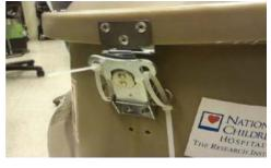
Correct (Below): Zip tie is connected to cryoport hood to prevent cryoport from opening
