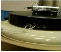
Incorrect (Below): Zip tie is not connected to cryoport hood
