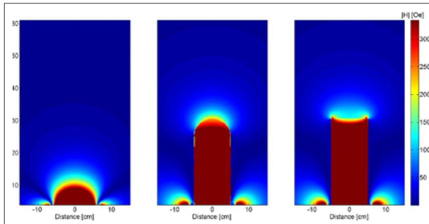
Calculated AMF distribution above a pancake coil without and with differently-shaped magnetic field concentrators.
