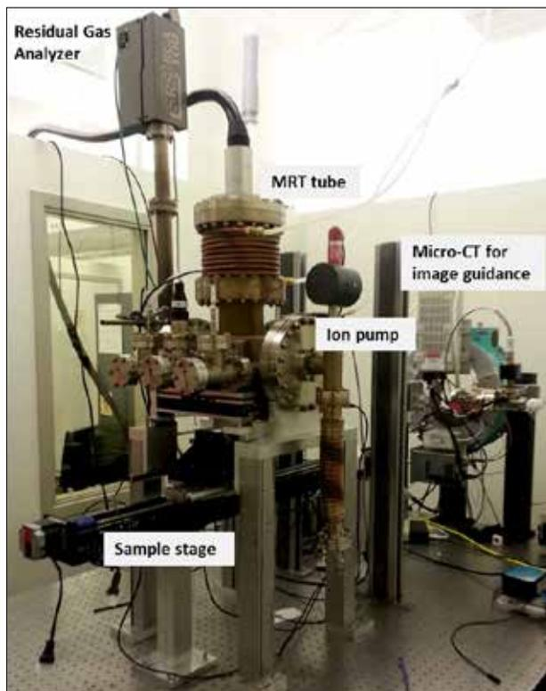
Picture of the desktop microbeam radiation therapy (MRT) system with integrated micro-CT mounted on the optical table.
