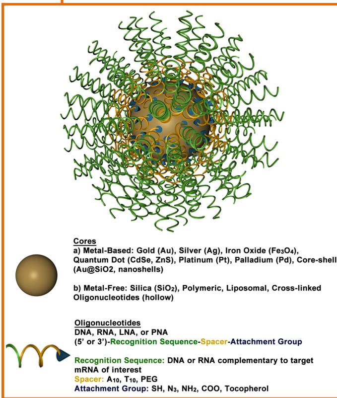
**Figure 3. Schematic representation of a Spherical Nucleic Acid (SNA) nanoconjugate.** The surface of a variety of different core materials including metal nanoparticles (e.g., Au, Pt), liposomes and polymers, can be functionalized with highly oriented nucleic acids (Reprinted with permission from Barnaby et al., 2015)<sup>54</sup>.
