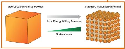
Figure 7. The Elan Nanocrystal™ technology.
